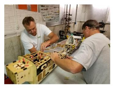
Once in the workshop, Mike and Mark methodically identified the path forward: the "ladders" structure that makes up the fuselage was really where the damage was. If we could get enough pieces glued back in, we could pull it back into alignment, then I could take it home and beef things up before finishing repairs.
