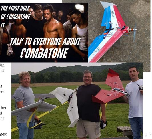
configuration that flies an 11x7 APC-style electric propeller. This means reasonable cost for servos, motors and ESCs. In fact, some guys are simply using their wrecked Parkzone T-28 innards to build Combat one, making it almost a free plane. Most guys are using the following or equivalent to handle their CombatONE:
