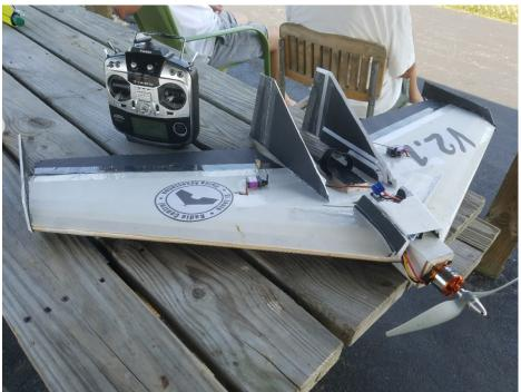
We've even been able to attempt a 3D version with rudders and a stabilizing 3D gyro... worked pretty good, but the knife edge could use some work!
