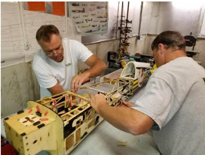
Once in the workshop, Mike and Mark methodically identified the path forward: the "ladders" structure that makes up the fuselage was really where the damage was. If we could get enough pieces glued back in, we could pull it back into alignment, then I could take it home and beef things up before finishing repairs.
